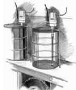
55 gallon (208 liter) drum mount on lubrication truck using drum cover
