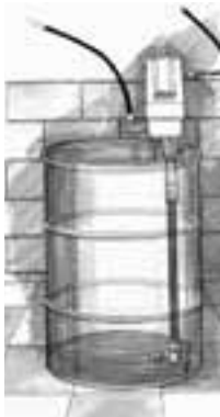
55 gallon (208 liter) drum mount using bung bushing
